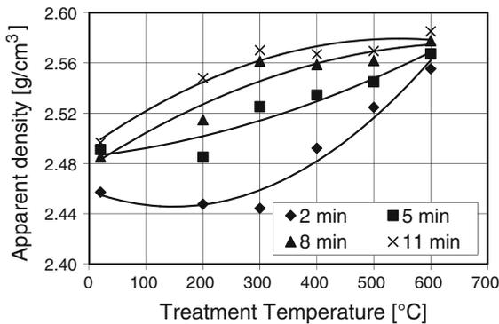
**Fig. 12** Influence of the treatment temperature and milling time on the apparent density of the coarse product (starting material 4/8 mm)
