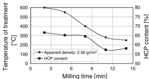
**Fig. 13** Combination of the milling time and the temperature for production the coarse products (input material 4/8 mm)
