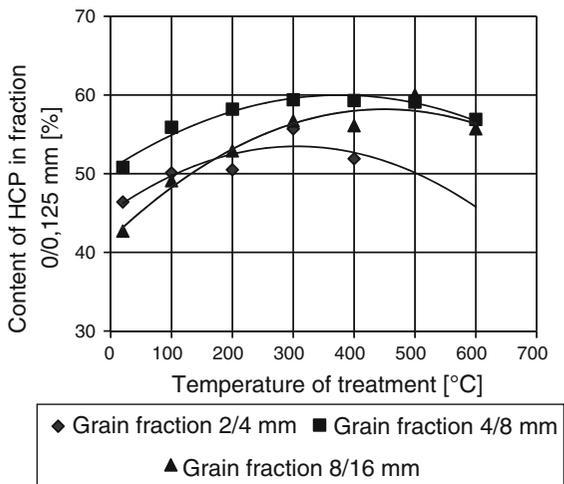
**Fig. 10** Influence of thermal treatment temperature on the content of HCP in the product 0/0.125 mm
