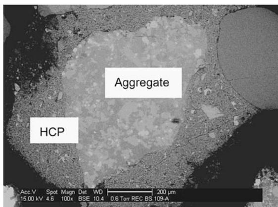
**Fig. 1** Layer of HCP at the surface of an aggregate grain (from [2])
