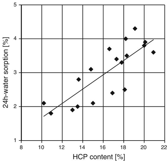
**Fig. 9** Water adsorption in dependence on the HCP content of the coarse products
