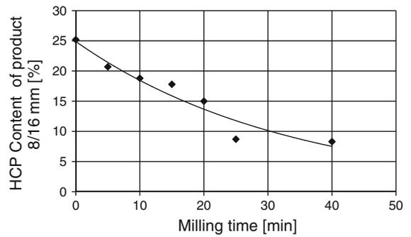
**Fig. 7** HCP content of the coarse products generated by mechanical treatment
