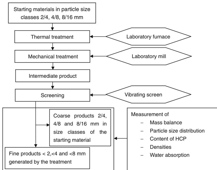
**Fig. 2** Procedure of the experiments
