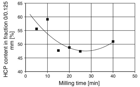
**Fig. 11** Influence of the duration of the mechanical treatment on the content of HCP in the product 0/0.125 mm
