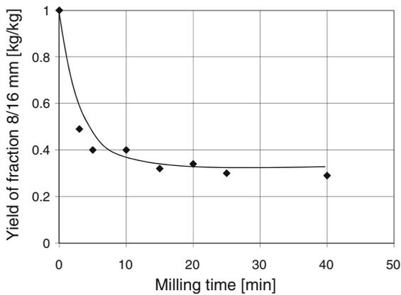
**Fig. 4** Influence of the duration of grinding on the yield of the mechanical treatment
