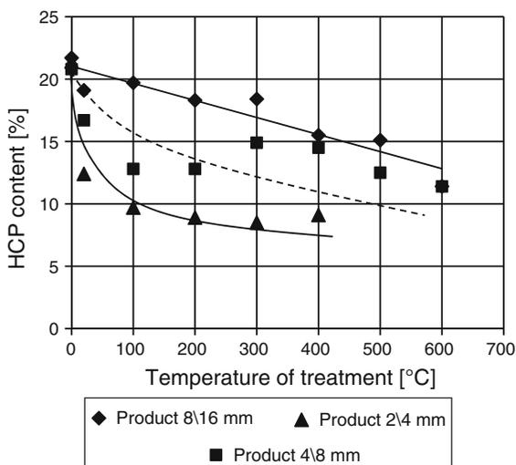
**Fig. 6** HCP content of the coarse products generated by thermal treatment (0 °C means: no treatment)
