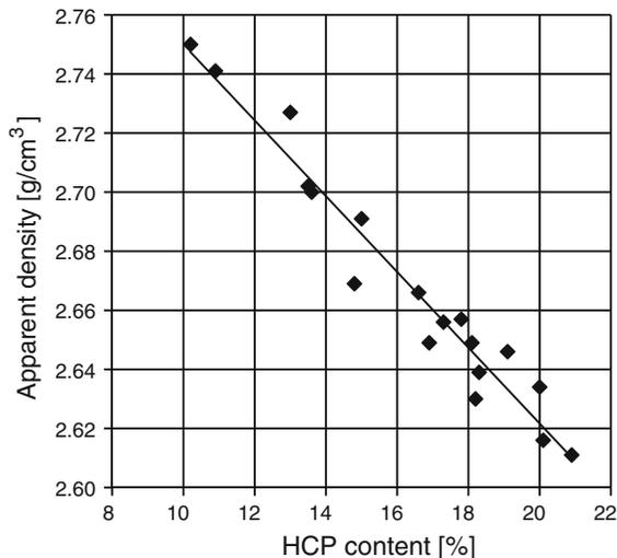
**Fig. 8** Apparent density in dependence on the HCP content of the coarse products
