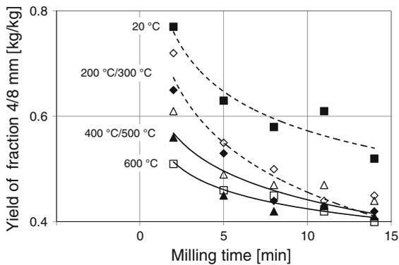
**Fig. 5** Influence of the duration of grinding and temperature on the yield
